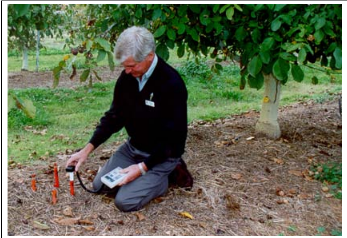
Plate 6. A tensiometer and digital readout used to measure soil water (matric suction).
